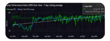
There is an initial improvement in the solar performance in January 2024, which aligns with the implementation of the PowerX platform. But soon after this, the SPR starts to regress.
